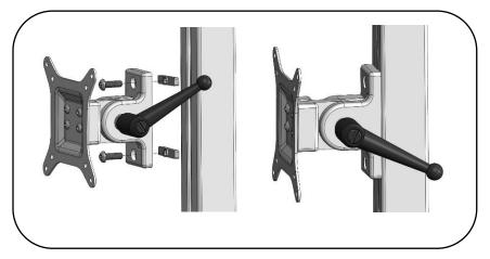
To move handle to a more desirable location; pull handle out, rotate CW or CCW and release handle. For locking handle operation see point 7.
