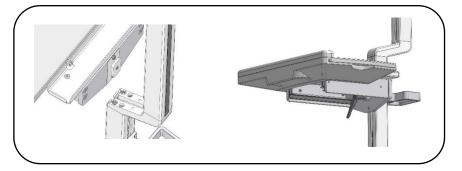
To move handle to a more desirable location; pull handle out, rotate CW or CCW and release handle (ref. point 6).
