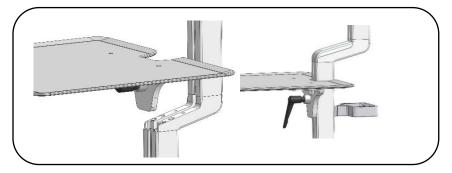
• To move handle to a more desirable location; pull handle out, rotate CW or CCW and release handle (ref. point 6).
