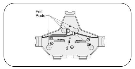
• Remove the 4 Screws holding the cover of the Universal Bracket using the 1/8-inch Hex L-Key from the front of the cover.
