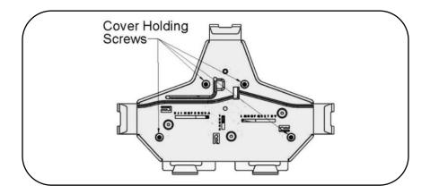
• Remove cover and the 3 screws holding the sliders using the 1/8-inch Hex L-Key from the front of the cover.
